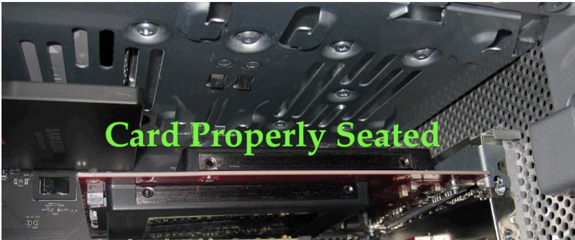
Figure 1: Inserting and securing the SeriTek/6G2+2 in a Computer
