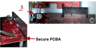
Tighten Screw to Secure Tab
