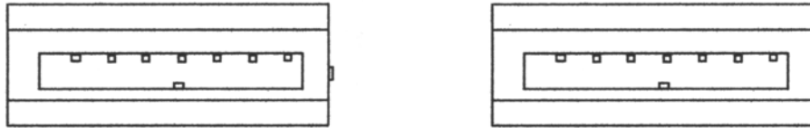
Figure 3: Using SeriTek/2SE4 with a drive enclosure that has L-shaped eSATA connectors; both cable connectors will be identical.
